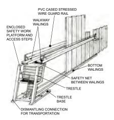
A complete tempory guide frame system to hold and support a panel of steel piles whilst they are installed. Guide walings are incorporated at two levels to provide precise guidance and support.
